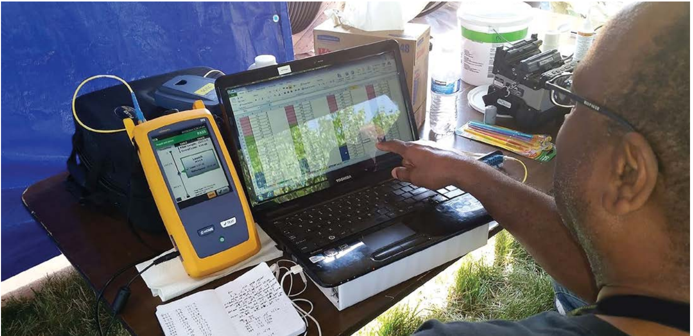
FIGURE 8: Testing an OSP spool of optical fiber. It is always recommended to test cables after delivery and compare the OTDR test results to the affixed test document on the spool.
